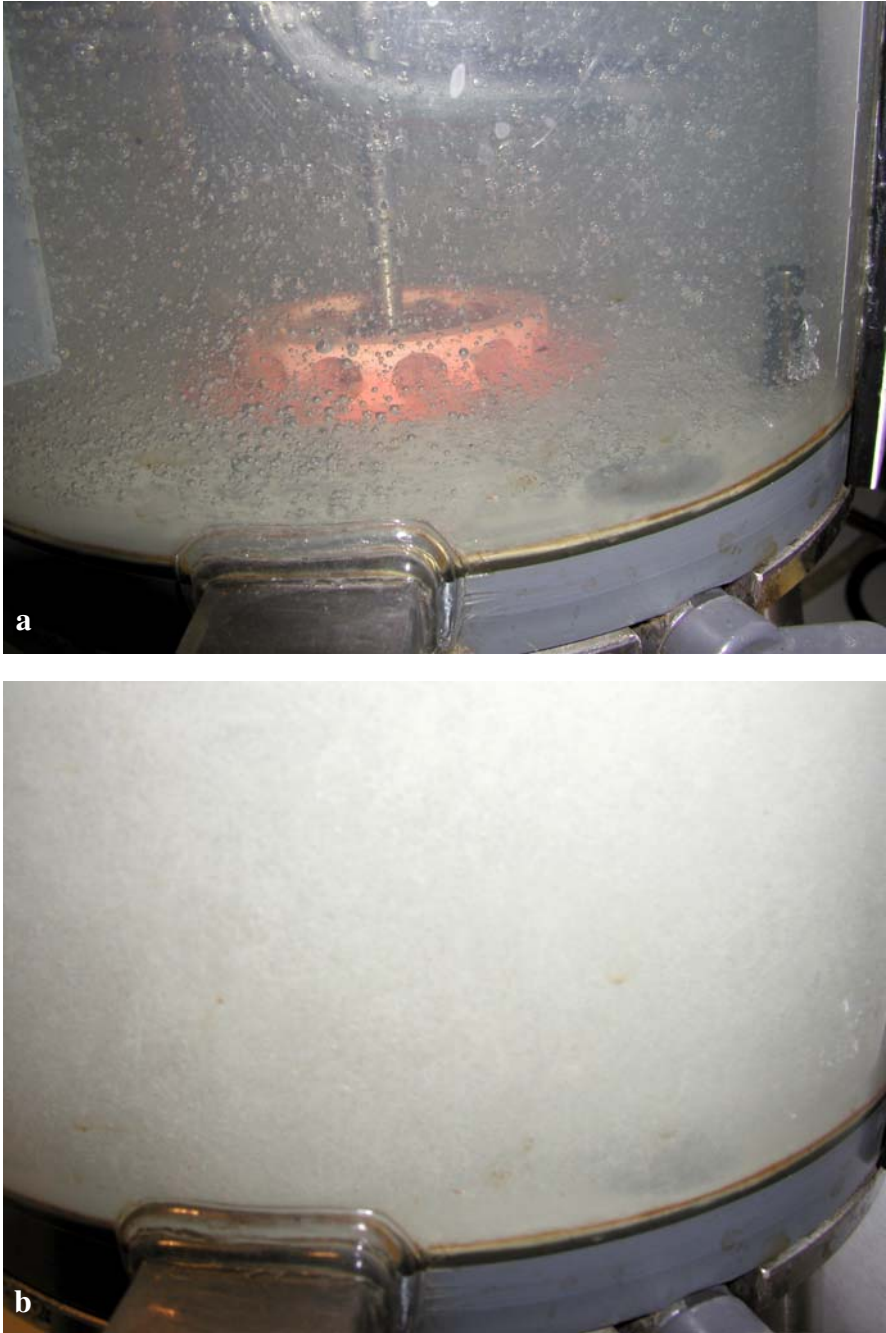
Figure 6.5 Photographs that demonstrate the coalescence phenomena in the same bioreactor (Frings 8-L) under similar conditions except for the ethanol concentration: a using tap water; b using an ethanol (1%) solution in water
