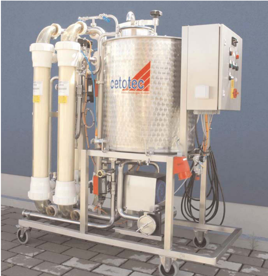
Figure 9.4 Model of a cross-flow filtration plant used for continuous microfiltration of vinegar
