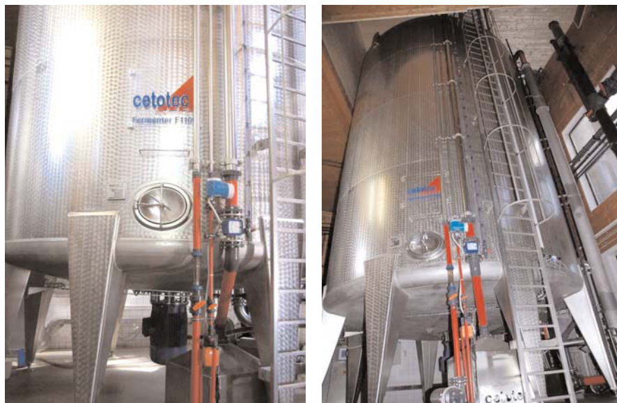
Figure 9.1 Example of a submerged vinegar fermenter with an annual production capacity of 18 million L of vinegar containing 10% acetic acid
