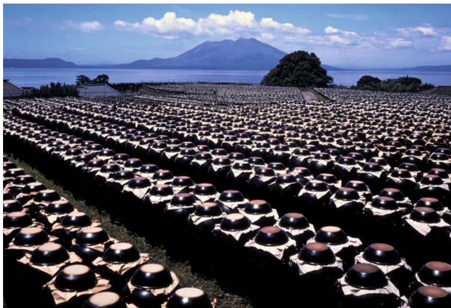
Figure 7.2 Traditional kurosu brewing in Fukuyama-Cho, Japan: ageing of kurosu using ceramic pot (picture provided by Sakamoto Brewing Co. Ltd.)
